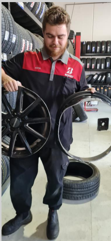
Justin holding up a wheel broken in half after hitting a large pothole.
